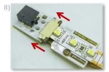
Secure the LED connector by closing the sliding latch. Again, the adhesive may want to resist. Your thumb nails are your friend here.
