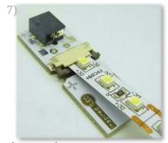
Make sure the LED strip is centered and fully inserted into the LED connector. You may need to hold the latch open with one hand so that the adhesive doesn't pull the latch closed prematurely.
